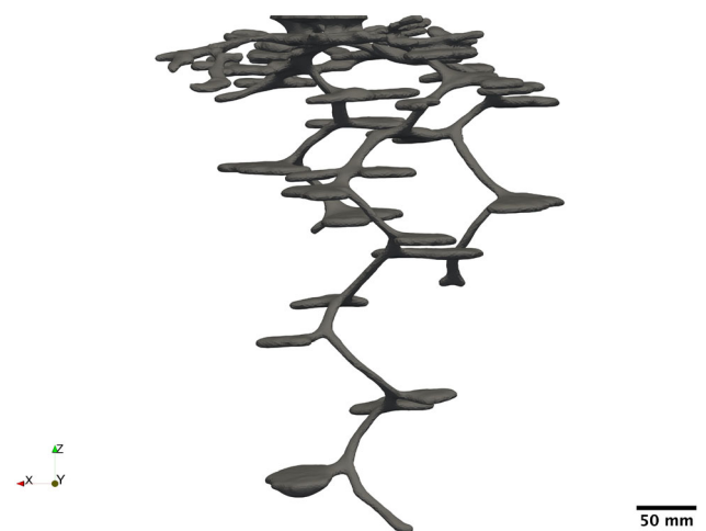
Fig. 3 3D image of the post-processed casting used as input to the FEM model
