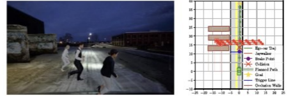
Fig. 5. Human Driving Failure Case: The one episode in which the human driver collided was the variation of Jaywalker with Occlusion scenario that involved multiple fast jaywalkers. The left image is captured at the braking point.
