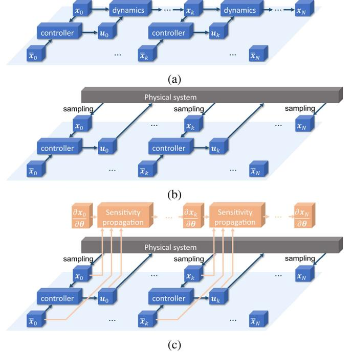
Fig. 3. Difference between a conceptual dynamical system (a) and a physical system (b). Since a physical system in (b) does not have a complete computational graph for autodifferentiation, sensitivity propagation is used for gradient computation and is illustrated in (c).
