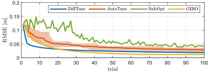
Fig. 4. Comparison of autotuning of Dubin's car using DiffTune, AutoTune [12], SafeOpt [9], and GIBO [43]. The shaded areas show the range of RMSEs (min to max) achieved in a total of 10 runs of algorithms that involve stochasticity (AutoTune and GIBO).
