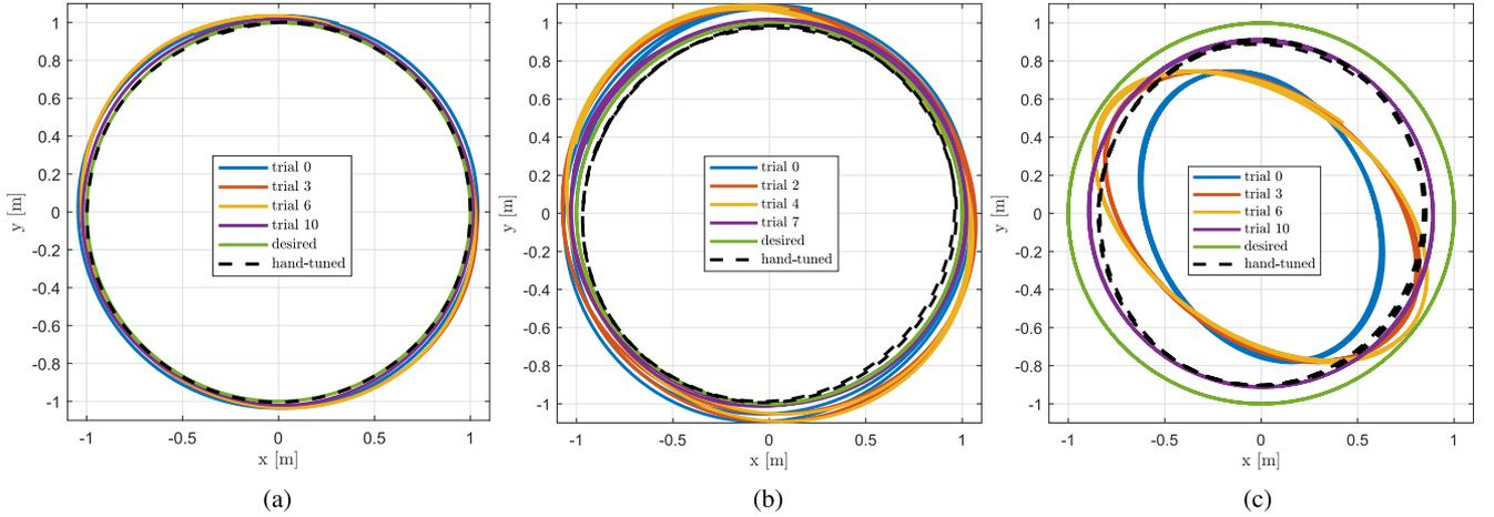
Fig. 9. Horizontal trajectories of the quadrotor during tuning on three circular trajectories with different speeds. (a) 1 m/s. (b) 2 m/s. (c) 3 m/s.
