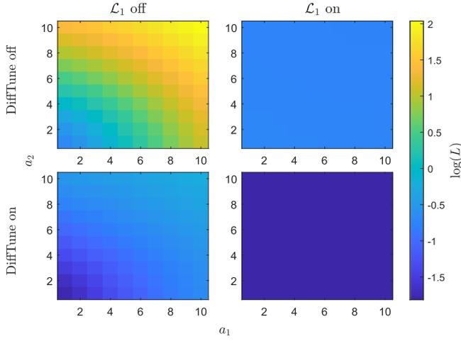
Fig. 6. Loss  $L$  subject to uncertainties (additive force  $0.1a_1 \sin(t)$  and moment  $0.1a_2 \cos(t)$  with  $a_1$  and  $a_2$  taking values from 1 to 10) in the ablation study of *DiffTune* and  $\mathcal{L}_1$ AC.
