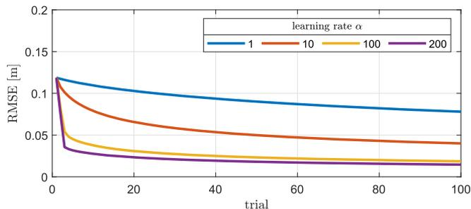
Fig. 12. Performance of DiffTune in Dubin's car example with different learning rates.
