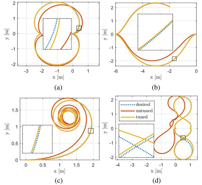
Fig. 5. Comparison of performance between tuned and untuned controller parameters on testing trajectories for generalization. (a) Peanut. (b) Lemon. (c) Spiral. (d) Twist.
