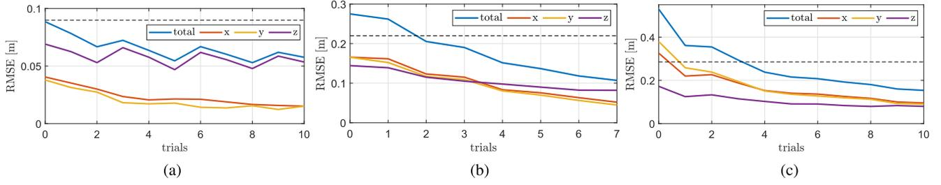
Fig. 8. Tracking error (RMSE) of the tuning on three circular trajectories. The dashed line shows the RMSE achieved by hand-tuning. (a) 1 m/s. (b) 2 m/s. (c) 3 m/s.
