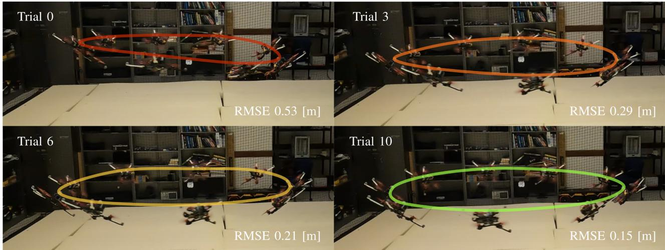
Fig. 1. Evolution of a quadrotor's tracking performance using DiffTune in ten trials [with  $3.5\times$  reduction on the root-mean-squared-error (RMSE)]. The quadrotor is commanded to track a 3 m/s circular trajectory ( $9\text{ m/s}^2$  centripetal acceleration). The tuning is conducted over 12 parameters. Video recordings of the four trials are available in the supplementary material.
