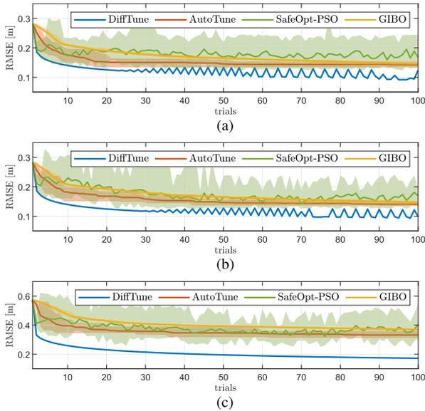
Fig. 7. Comparison of tuning the controller of a quadrotor using DiffTune (proposed), AutoTune [12], SafeOpt-PSO [31], and GIBO [43]. The shaded areas show the range of RMSEs (min to max) achieved in a total of ten runs of the algorithms that involve stochasticity (AutoTune, SafeOpt-PSO, and GIBO). (a) 2-D circle. (b) 3-D circle. (c) 3-D lemniscate.
