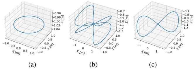
Fig. 15. Trajectories used in the generalization test. (a) Circle. (b) 3-D lemniscate. (c) Vertical lemniscate.
