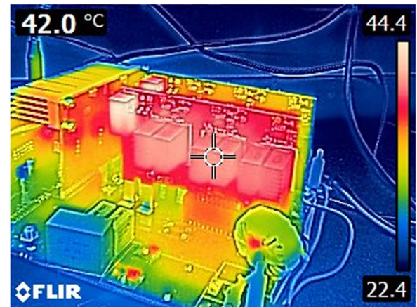
FIGURE 22. Thermal image of the converter operating at 1.25kW for input voltage V_{AC} = 120\text{Vac rms} .
