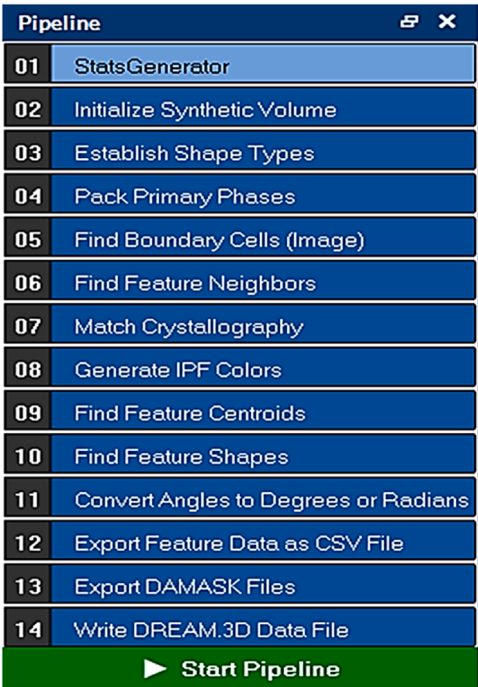
Figure A1. DREAM.3D pipeline for generating the RVE.
