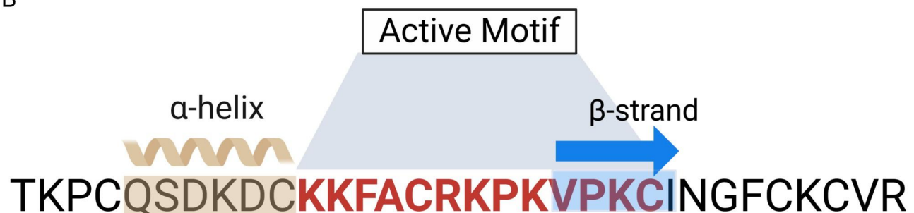
Fig 6. Active motif of NCR13 required for antifungal activity. (A) Antifungal activity of reduced NCR13_CS and reduced NCR13 alanine variants against B. cinerea . Alanine scanning mutagenesis was done by substituting alanines within the NCR13 core sequence, leading to the creation of the NCR13_AlaV1-V5. MIC values and net charge of all peptides were determined. The amino acid substitutions that completely inactivate the peptide are shown in red. Representative pictures are shown in the S6 Fig. (B) Active motif of NCR13 (highlighted with a bold red font) required for its antifungal activity against B. cinerea . The secondary structure elements are shown above the amino acid sequence. The brown wavy symbol and blue arrow indicate \alpha -helix ( \alpha 1) and \beta -strand ( \beta 1) respectively.
