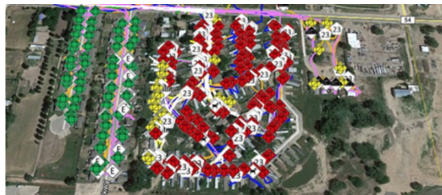
Figure 1: A map annotated with standard GPS waypoint markers during SAR operations, which enables collaborative planning of operations and real-time sharing and tracking of plans.
