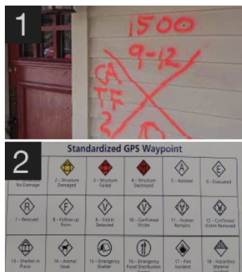
Figure 4: Different methods of the marking system used to keep track of the SAR operation plan: (1) Spray painting buildings. (2) Standardized GPS waypoints used in digital maps (see Figure 1).
