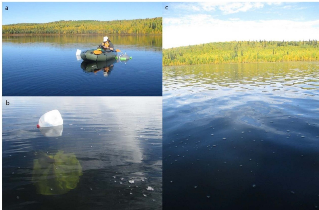
Figure 5. September 2021 field observations at N. Blair L. included flux measurements with a floating chamber attached to a LGR-ICOS microportable greenhouse gas analyzer (a), bathymetric measurements, and collection of gas samples with underwater bubble traps (b). Active bubbling is seen on lake surface (b), (c) and was mapped at the location of the high L-band SAR backscatter anomaly. No evidence of oil or oil slicks were seen at NBL. (a) Photo reused with permission from Peter Anthony. (b), (c) Photo reused with permission from co-author Katey Walter Anthony.
