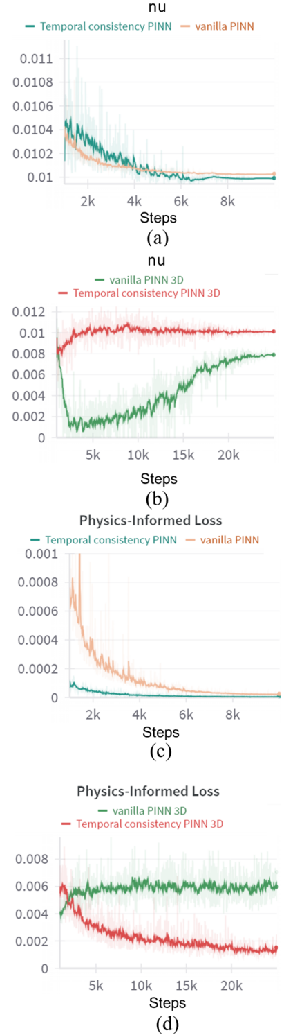
FIG. 5. Comparison of convergence of viscosity for the (a) two-dimensional and (b) three-dimensional Navier-Stokes equations between vanilla PINN and PINN with temporal consistency. While for the 2D case, the vanilla PINN converges to a very similar value for viscosity, for the 3D case, the prediction of the temporal consistency PINN is more accurate to the ground truth value of 0.01018. The better convergence of the temporal consistency PINN can be further demonstrated using the physics-informed loss term for the (c) 2D and (d) 3D cases. While the temporal consistency loss term converges faster for both cases, for the 3D case, it does significantly better than vanilla PINN.
