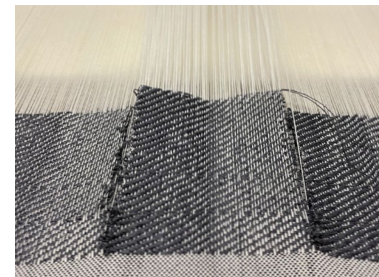
④ Weave draft provided to the loom. ⑤ Partial-weft fabric on the loom. ⑥ Resulting fabric, woven in one piece with no cutting.
