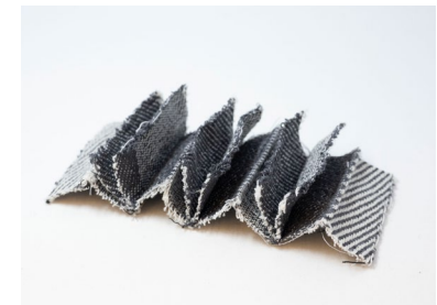
④ Weave draft provided to the loom. ⑤ Partial-weft fabric on the loom. ⑥ Resulting fabric, woven in one piece with no cutting.
