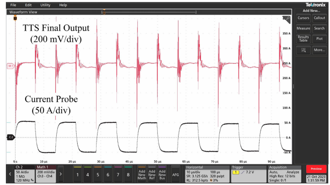
Fig. 6. Design I test results for 50 A peak-to-peak 70 kHz current pulses.
