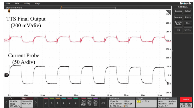
Fig. 13. Design IV test results for 50 A peak-to-peak 70 kHz current pulses.
