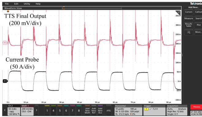
Fig. 11. Design III test results for 50 A peak-to-peak 70 kHz current pulses.
