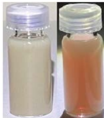
Figure 1. Dichroic colloidal solution of silver nanoparticles in reflected light (left) and transmitted light (right)
