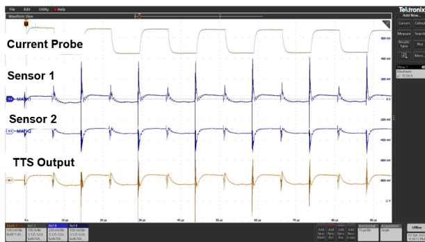
Fig. 6. Test result for validating TTS solution on the slitted trace
