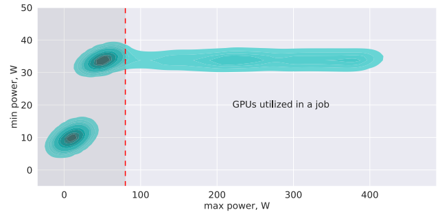
Figure 7: Distribution of GPU power consumption extrema in individual jobs. Dashed line at 80W shows the cut-off value to deem GPUs utilized by the job.
