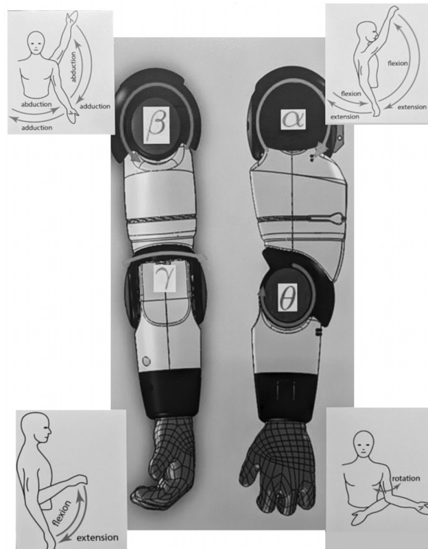
Figure 5. Zeno's arm with its four degrees of freedom [29].
