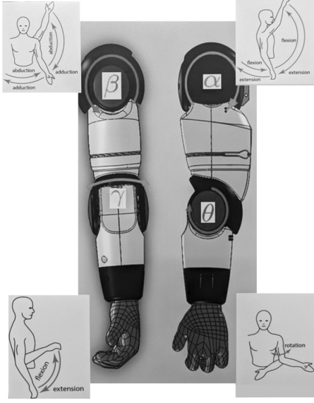
Fig. 6: Zeno's arm with its four degrees of freedom [27].
