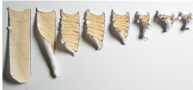
Left: S twist yarns; right, Z twist yarns. Twist angles of 5–40° in 5° increments. The Z twist yarns are animated at a lower twist angle, because only Z twist single yarns have been used – in the S twist yarns, some energy is lost as the Z twist singles are twisted in the opposite direction during plying.
