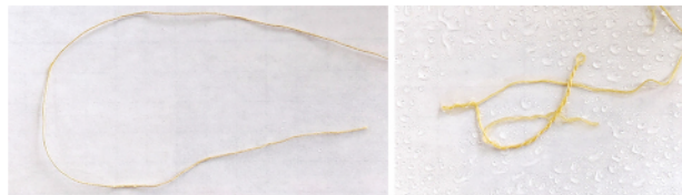
Nm 21/3 25° Z twist yarn when dry (left) and wet (right).
