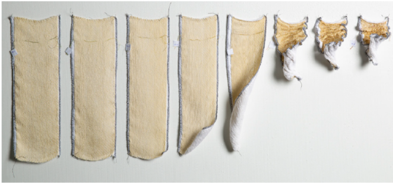
Left: S twist yarns; right, Z twist yarns. Twist angles of 5–40° in 5° increments. The Z twist yarns are animated at a lower twist angle, because only Z twist single yarns have been used – in the S twist yarns, some energy is lost as the Z twist singles are twisted in the opposite direction during plying.
