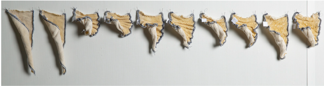
Weave structure float length. Left to right: 0.8 mm, 1.3 mm, 2.1 mm, 2.9 mm, 3.8 mm, 7.9 mm, 9.6 mm, 12.1 mm, 14.2 mm, 17.1 mm. Yarn: Nm 21/3 20° Z twist.
