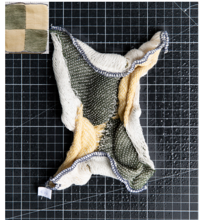
The sample with S (green) and Z twist (yellow) yarns in a checked pattern showing uneven yarn energy when activated, producing a new animated morphology. Inset: before activation.
