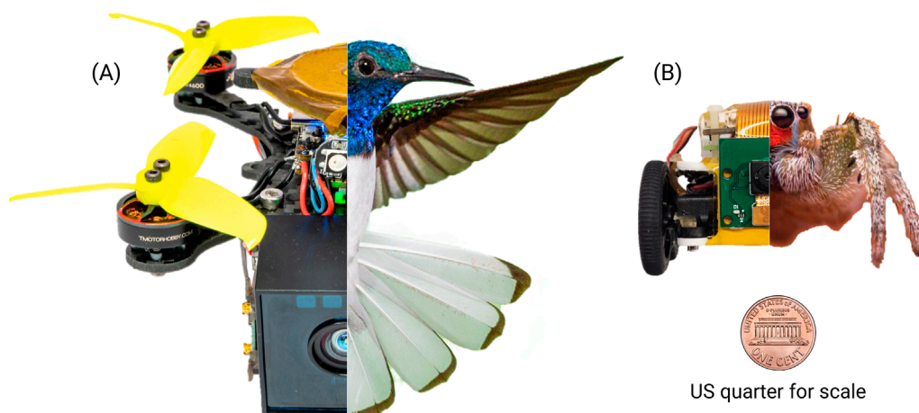
FIGURE 1 Tiny autonomous robots that utilize our Minimal Perception framework. (A) Autonomous drone of ~120 mm in diagonal length and compared with hummingbird. (B) Autonomous car of about ~70 mm in length and compared with a wolf spider.
