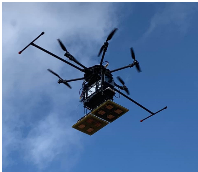
Fig. 1. Radiometer integrated on a custom UAS.
