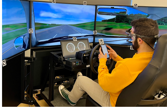
Fig. 1. Participant is wearing the eye tracker and performing NDRTs on a smartphone while the vehicle is in automated driving mode.
