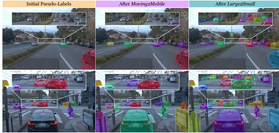
Fig. 2: Visualization of pseudo-labels at each stage of our self-training paradigm. From the initial pseudo-labels L_i^{(0)} generated from motion mask, L_i^{(1)} retrieves the large static objects after Moving2Mobile and L_i^{(2)} recovers the small objects after Large2Small .
