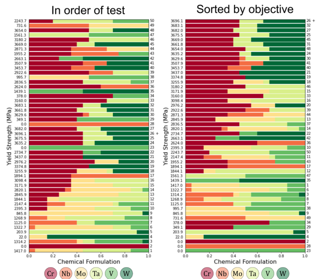
Fig. 7 Compositional color bar map of compositions in Fig. 6, organized by test order and by property order. The maximum is noted with a '+'. It is evident from the left panel that the BO scheme first investigates Cr-rich alloys, then alloys that are rich in Cr and W, and finally begins exploring the space in later iterations. Specifically, the BO scheme investigates alloys that are more rich in Mo. In the right panel where alloys are sorted by objective it is evident that Cr-Ta-W ternaries have the highest yield strength according to the Maresca-Curtin model.
