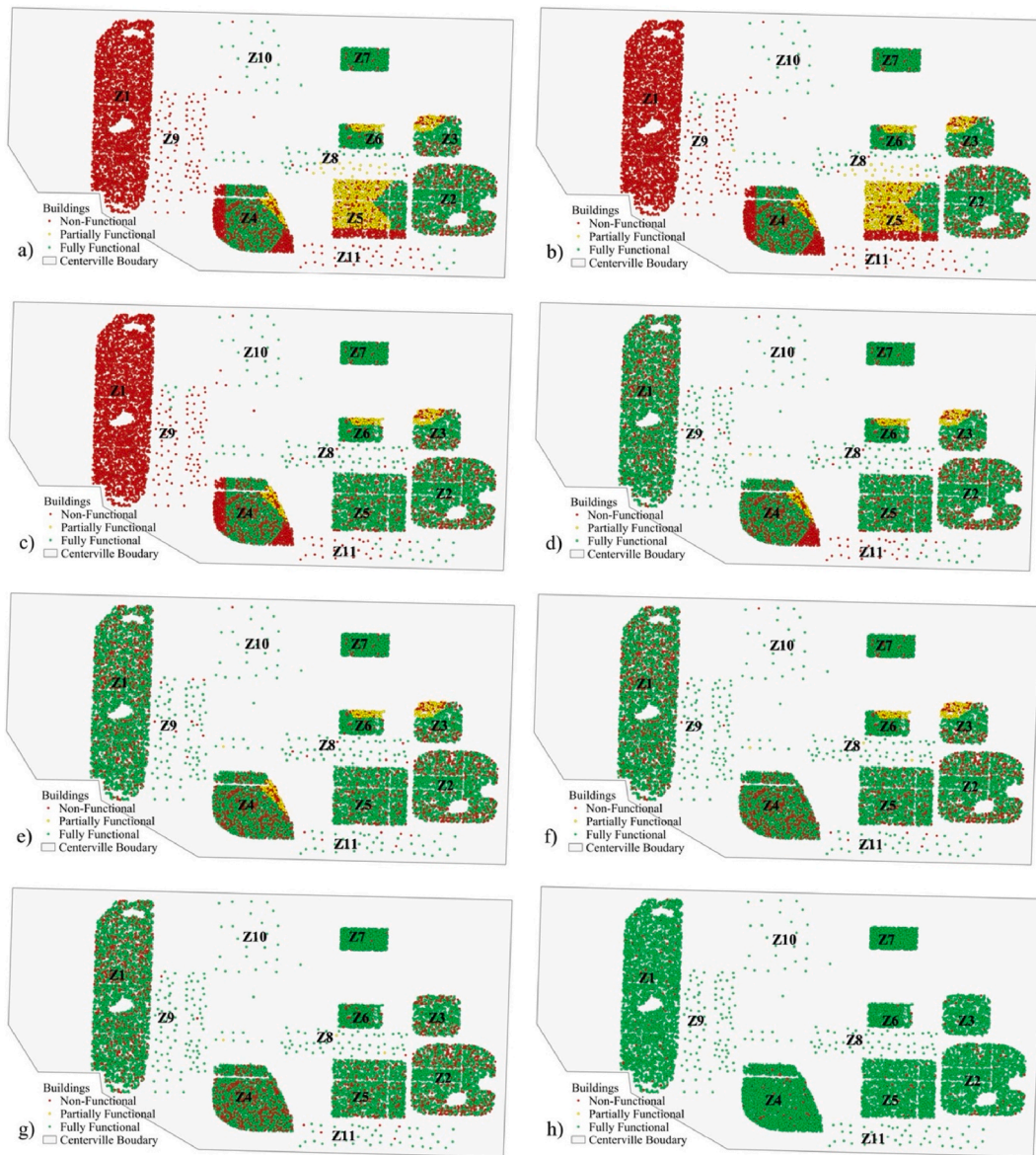
Fig. 13. Functionality of buildings after: a) the earthquake, b) 3.02-days, c) 6.1-days, d) 7-days, e) 14-days, f) 75-days, g) 220-days, and h) 900-days.
