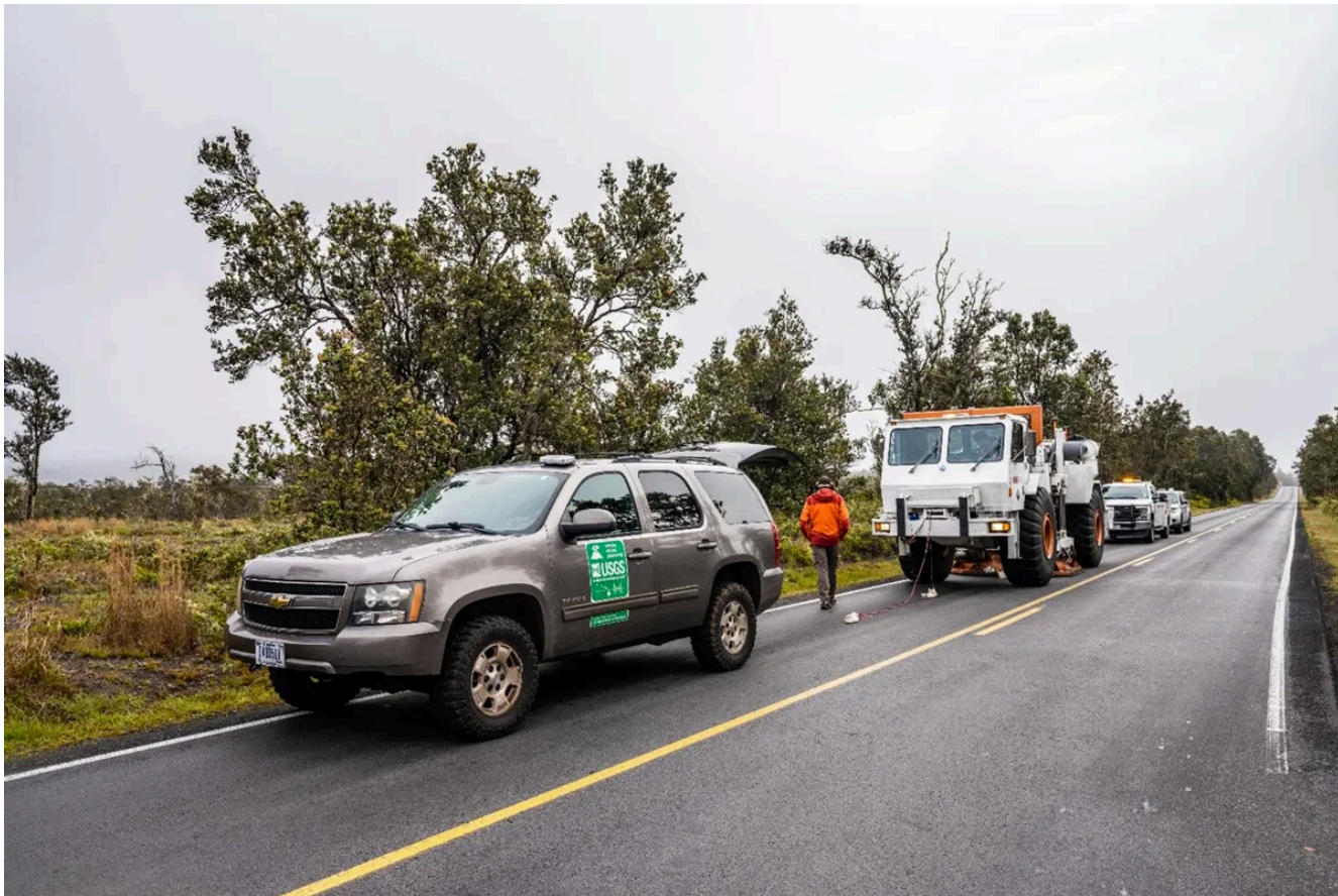
The T-Rex vibroseis source operates along Crater Rim Drive just northeast of the abandoned U.S. Geological Survey (USGS) Hawaiian Volcano Observatory (HVO) building and the closed National Park Service Jaggar Museum. T-Rex and its USGS support vehicle (foreground) are flanked by two vehicles for traffic control. Roger Denlinger of USGS walks toward T-Rex after placing accelerometers on the pavement to monitor the intensity of the shaking. If the local ground vibration exceeded a threshold recommended by Hawaii Highway Division engineers, shaking was immediately stopped. Credit: Janice Wei/National Park Service
