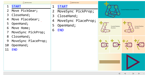
Figure 1: RobotStudio Online YuMi programming interface for two-armed robots: Two canvases show RAPID code for each arm side-by-side, with buttons allowing the quick insertion of commands into the code.
