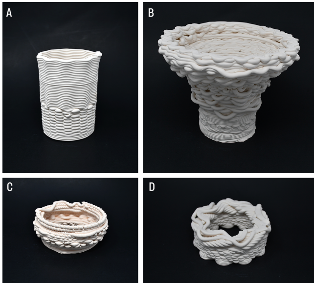
Figure 6: Pieces produced through the rapid and irregular tuning of texturizer parameters.
