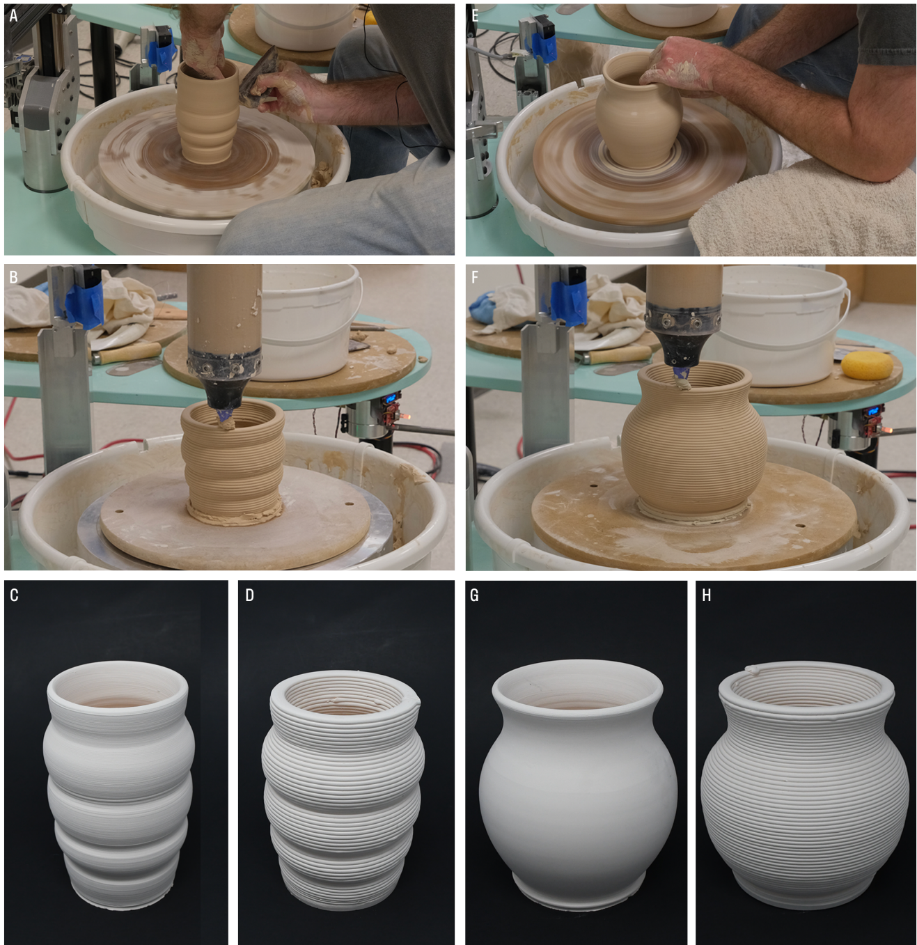
Figure 8: Workflow of scanning and printing pieces thrown on the wheel. A) Isaih throwing a mug on the wheel by hand. B) Thrown mug being 3D printed on the wheel from a scan of the original mug. C) Thrown mug. D) Printed mug. E) Isaih throwing a vase on the wheel by hand. F) Thrown vase being 3D printed on the wheel from a scan of the original vase. G) Thrown vase. H) Printed vase.
