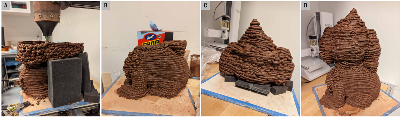
Figure 17: The fabrication process of Eun-ha's Obsidian poodle shown in Figure 1E. (A) Printing with foam supports for overhangs. (B) The poodle's head did not survive the print, leaving only the body. (C) Eun-ha printed the head separately. (D) The parts were manually attached together.
