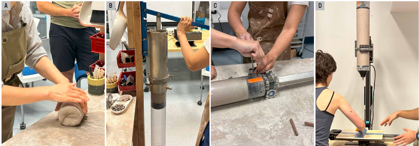
Figure 16: PotterBot tube loading workflow. (A) Eighteen pounds of clay gets wedged and shaped into a tube-sized cylinder. (B) Wedged clay gets loaded into the wall-mounted extruder and compressed into the PotterBot tube. (C) Sixteen screws are screwed to attach the motor to the top of the tube and the nozzle to the bottom. (D) The tube gets hefted into the PotterBot's z-axis clamp, and the bed is prepped.
