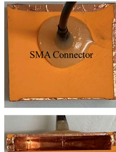
Fig. 9. Side view and front view of the waveguide probe.
