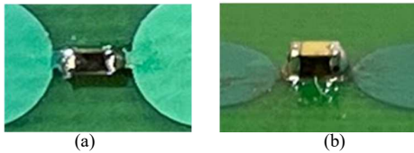
Fig. 5. Two orientations for MLCC soldering. (a) Black side facing the top side. Applied in round 1 and round 3. (b) Black side facing the front side. Applied in round 2 and round 4.
