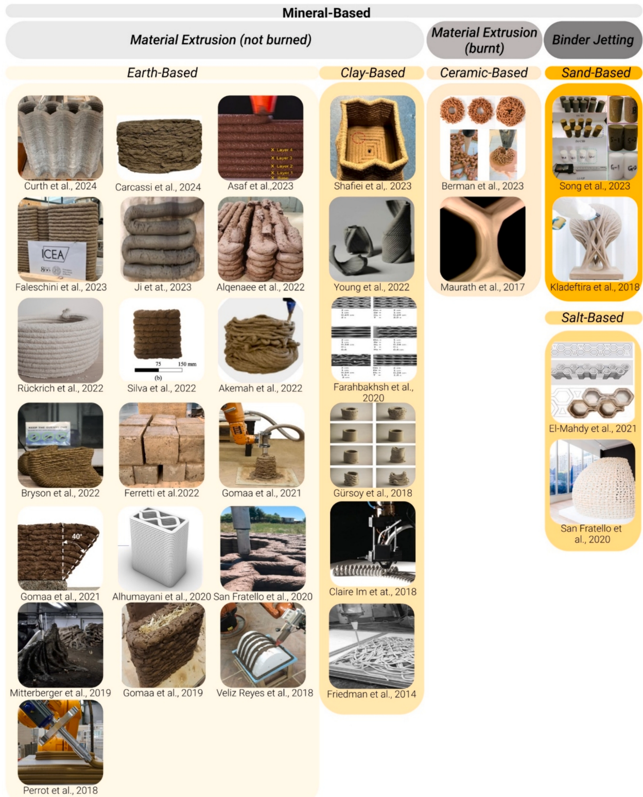
Fig. 4. Mineral-based research papers categorized according to the AM technique (material extrusion (ME) and binder jetting (BJT)) and the main material sub-category (earth-, clay-, ceramic-, sand-, and salt-based).
