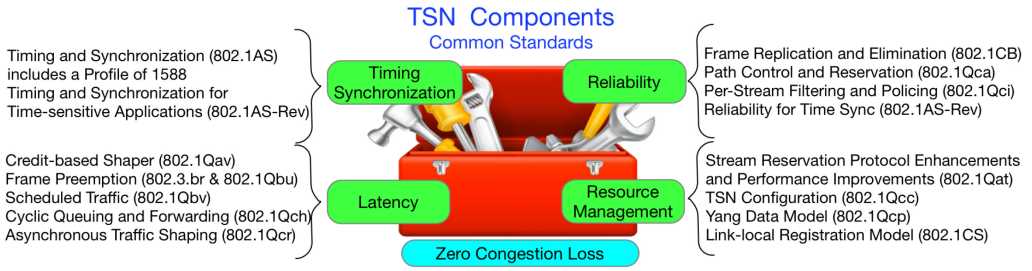
Fig. 3. IEEE 802.1 TSN toolbox, consisting of four coarse subclasses. Some draft standards (e.g., IEEE P802.1ASdm and IEEE P802.1Qdj) are still in progress and thus are not included in the discussion in Section 5.
