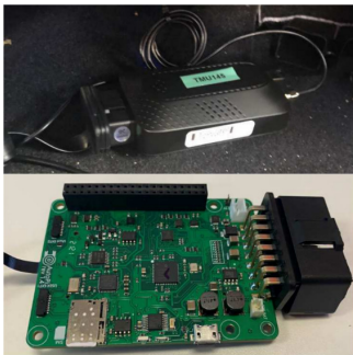
FIGURE 9: AutoPi device used for collecting telematics data, including speed, SOG, azimuth, distance, and GPS coordinates [26], [27].
