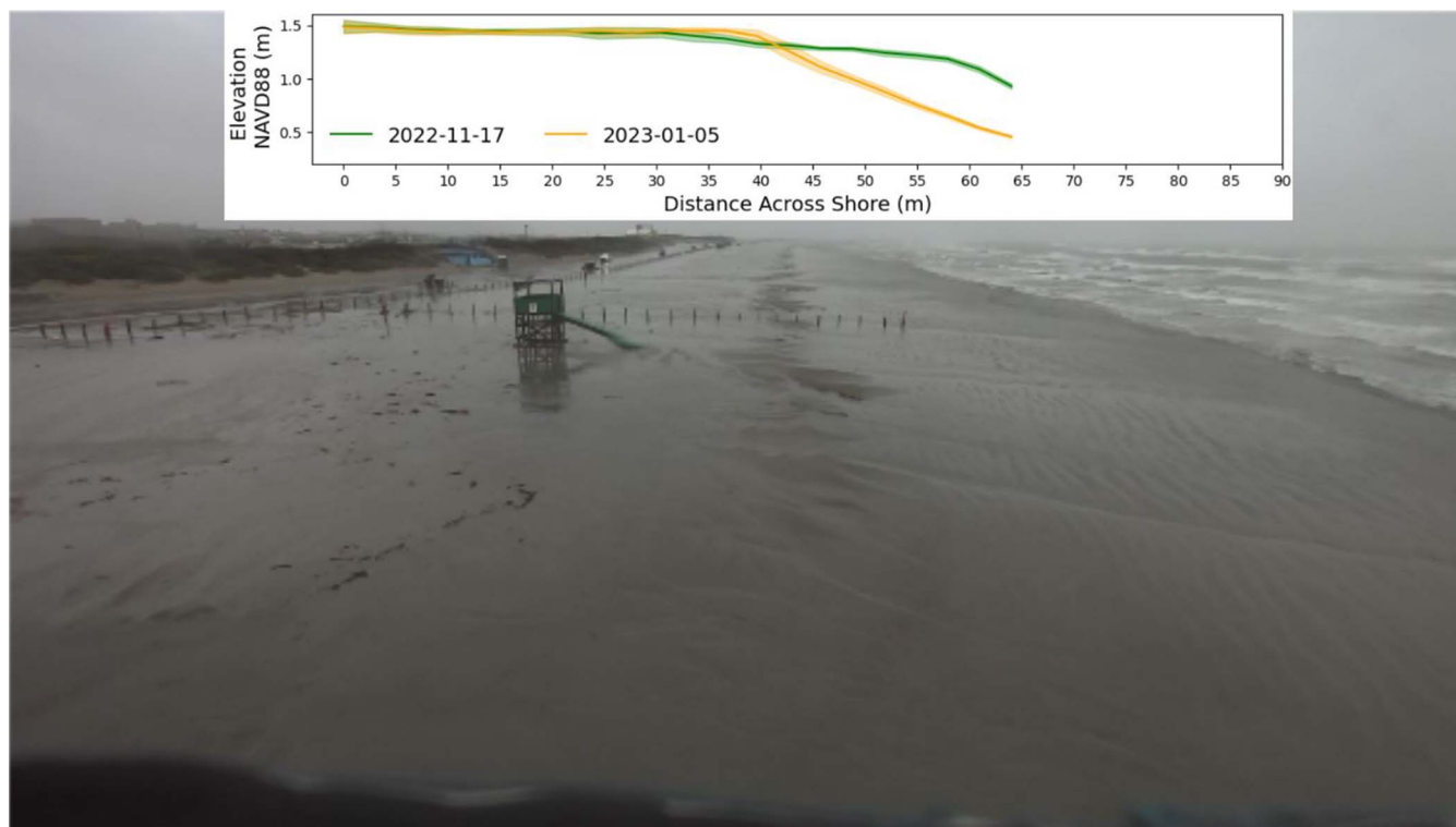
Figure 9. Inundation event on 19 November 2022 (1400 [central daylight time]). The beach profile at the top of the figure illustrates the foreshore erosion consistent with the long, dominant wave period.
