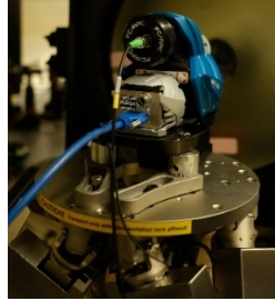
Fig. 14. HASO LIFT 680 Shack Hartmann sensor assembly integrated with PI H-824 hexapod positioner at the back focal plane of the telescope.
