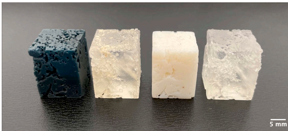
Fig. A.7. Photograph of the produced printed soil analogues by DLS, PJ Gel, PJ WS, and LFS arranged left to right.
