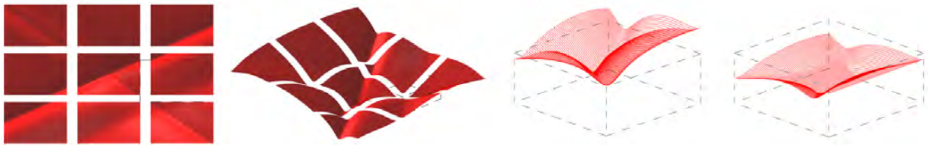
Figure 5: Milling Subsets of the Goldstein-Price Function in the D2: FunctionTile notebook. 1) Top-down view of a surface rendering of nine subsets surrounding the global minimum of the Goldstein-Price function. 2) An isomorphic view of the same rendering. 3) Toolpath rendering of the single subset containing the global minimum (center of the nine), currently infeasible to mill due to the toolpath lying almost entirely above the material. 4) After interactively processing the toolpath by dividing the function output, adding a vertical offset, and clamping the function to a desired bounds, the toolpath becomes feasible to mill into a mold.
