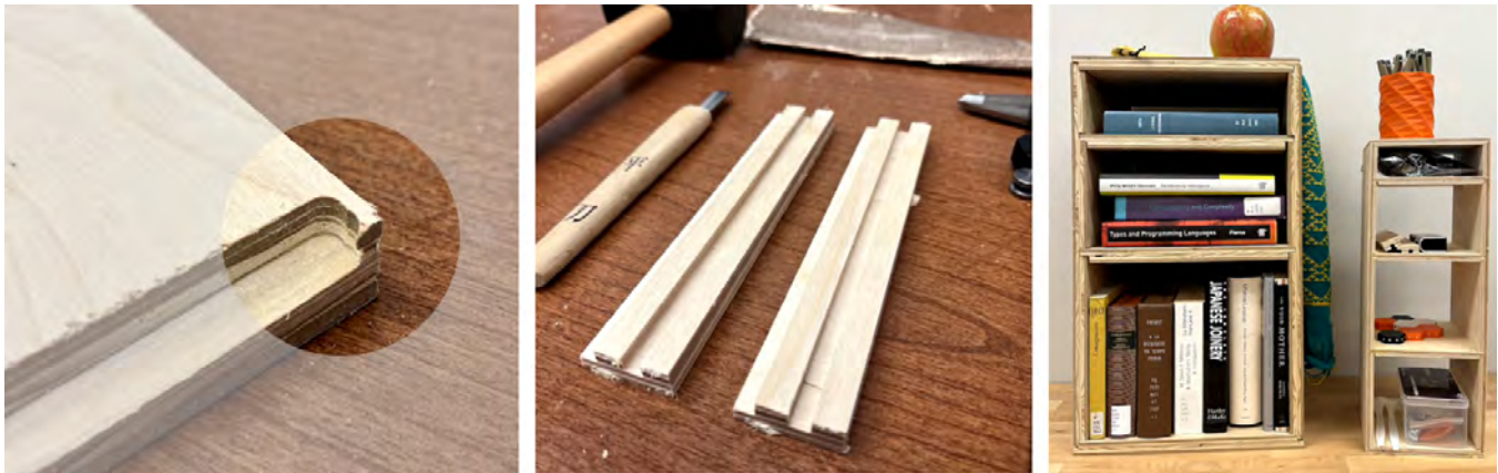
Figure 12: Moments from Developing MiniShelf. Left: a miscalculation in generating the rabbet toolpath left artifacts in the corners. Middle: parametrically generated test pieces to check the cut depth of the joints. Right: two shelves each fabricated with MiniShelf.
