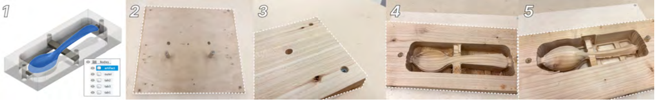
Figure 6: Moments from Siena’s Steps in the Notebook. (1) Given the already modeled spoon, Tandem generates the outer and tabs that surround the spoon. (2) A completed alignment jig. (3) The main workpiece S_{main} after being milled to the height of the spoon a_z . (4) The top face F_A of the main workpiece S_{main} after milling the top-down cut. (5) The bottom face F_B of the main workpiece S_{main} after milling the bottom-up cut.
