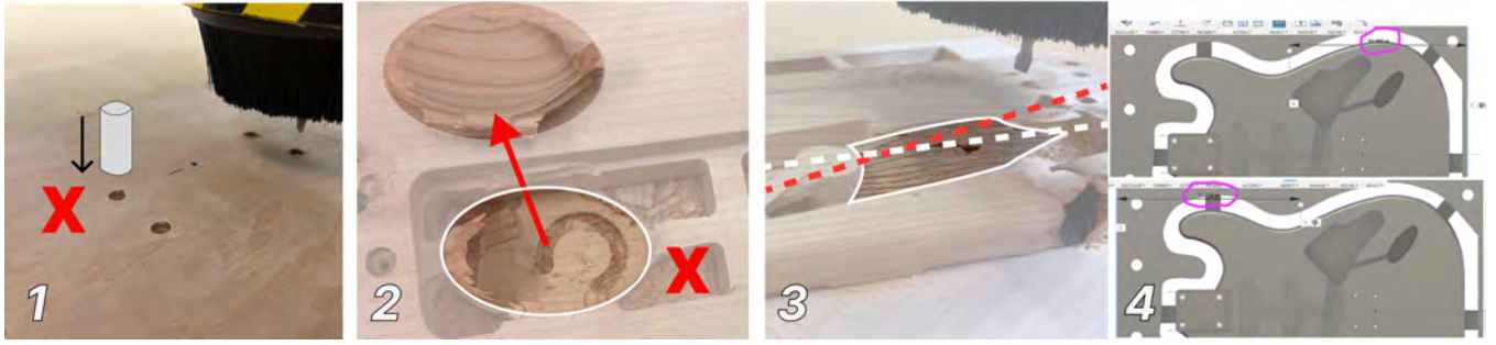
Figure 3: Examples of Errors that Arise in Two-Sided Milling. (1) A milled alignment hole is too narrow for the dowel to fit, requiring a second set of holes to be milled. (2) The CAD design of a spoon features a handle that is too narrow and gets torn off by the mill. (3) Flipping the workpiece over an axis that deviates too much from an assumed axis of rotation results in an invalid post-milling geometry. (4) An error taken from an online forum [64] where a fabricator reported misaligned features while milling a guitar. Another forum user responded that the reason was that the alignment holes were asymmetric across the axis of rotation assumed by the original poster.
