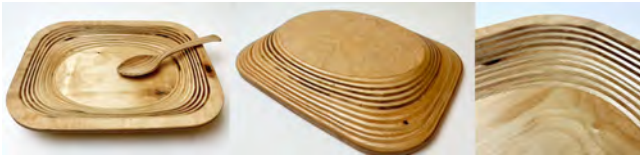
Figure 21: A Bowl Milled from a Stack of Plywood. Because the bowl is ellipsoidal, it cannot be turned on a lathe and must be milled.
