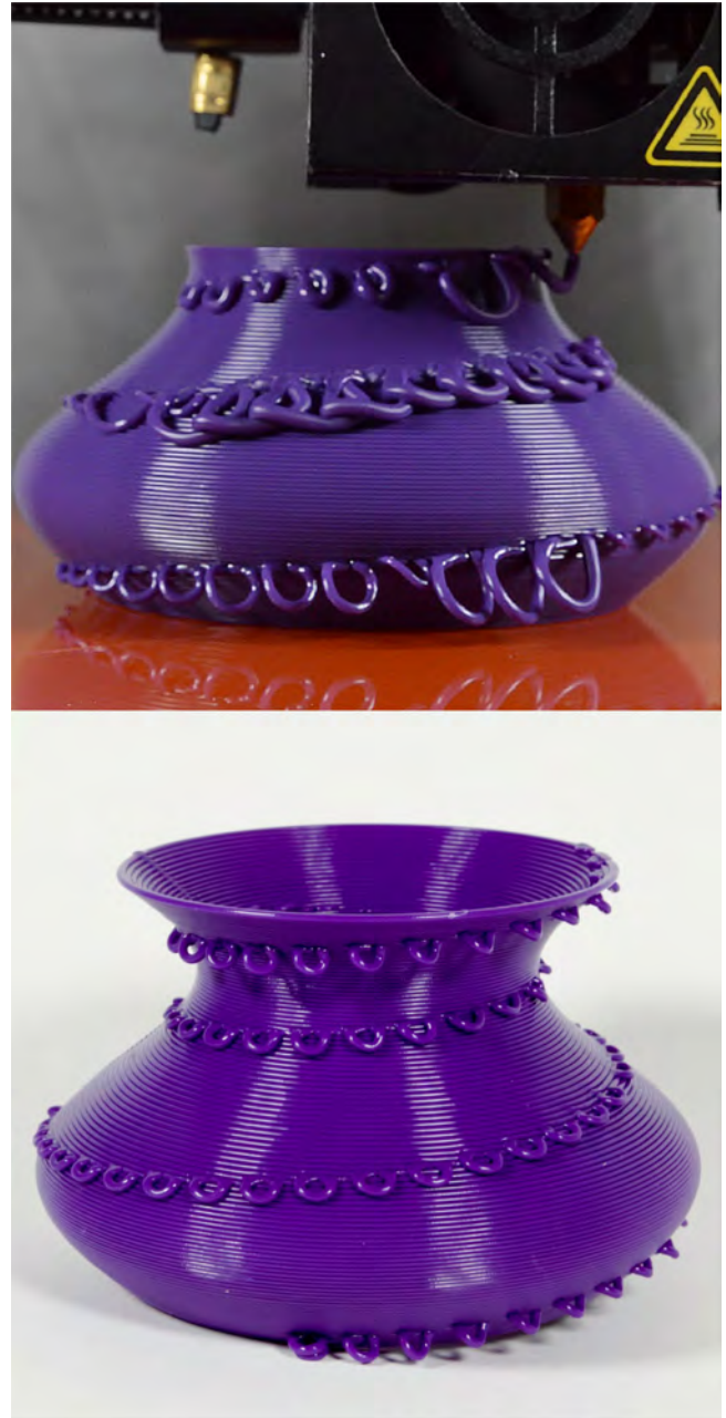
Figure 2: (Top) Exploring loop parameters with our MIDI-interface. Loop radius, extrusion, and speed are varied during execution to understand the material response. (Bottom) After exploring a variety of loop shapes and sizes, we can commit to fabrication with desired parameters. Shown is an image of a print with constant loop settings, determined through previous exploration.
