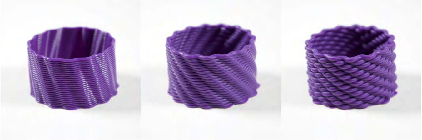
Figure 3: Our approach can be applied in a variety of contexts. In the prints shown, speed, extrusion quantity and toolpath geometry are modified to catalog a variety of woven textures.
