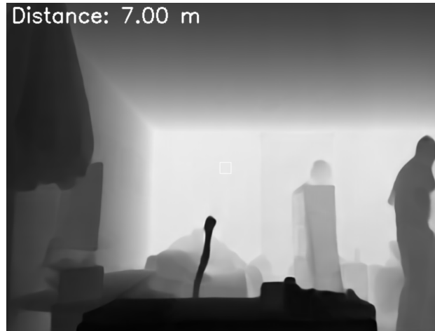
Fig. 7 Depth map generated from Metric3Dv2 output with distance from the center pixel overlaid.
