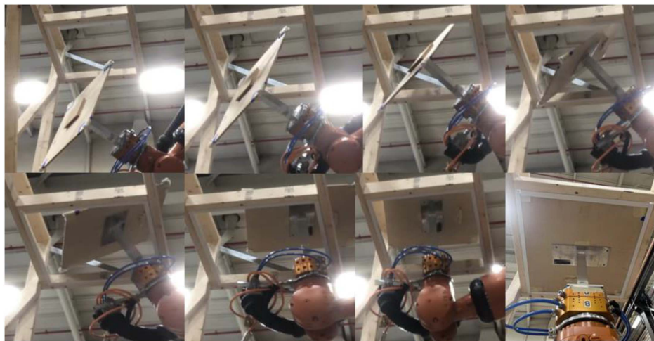
Fig. 10. A KUKA KR120 robot following the demonstrated motion primitives.
