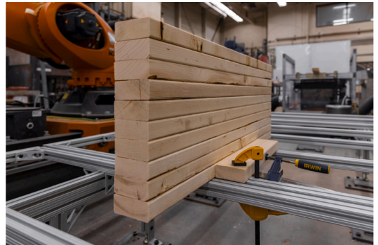
Fig. 9. The adaptive experimental scenario, with both robots alternating to assemble an NLT panel using the developed pose-based adaptive fabrication method.
