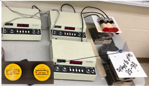
Fig. 1. (a–b). (a) Setup for gamma radiation measurement along with radiation sources (Cs-137); (b) Internal circuitry of the nucleus 500 digital radiation counter.
