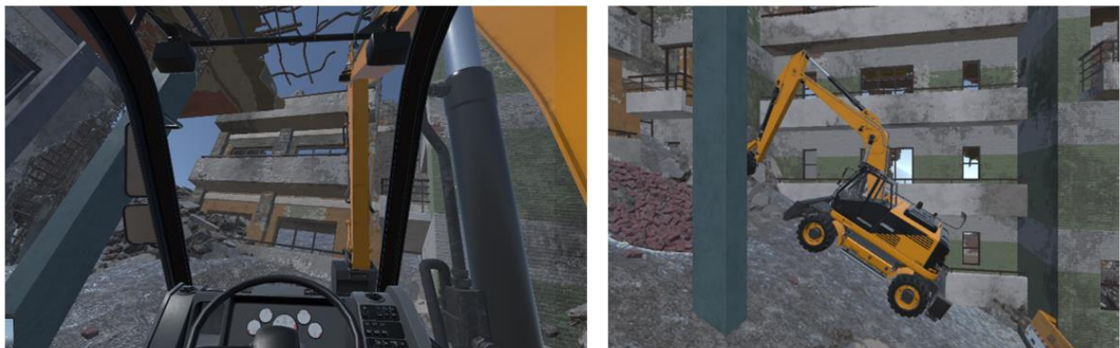
Figure 3. Example images of distorted axis in 1st person view (left) compared to the 3rd person view from an uneven and sloping jobsite (right)
