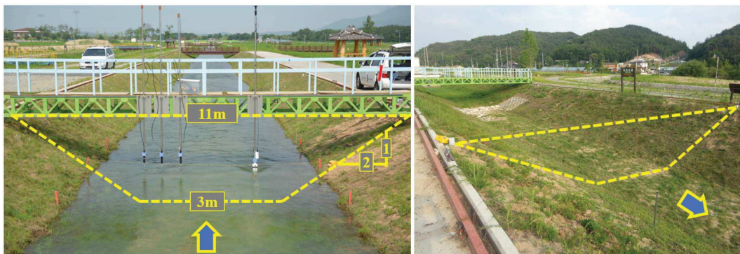
Fig. 5. Flume specifications and images of the experimental channel used in the study. (Image by Jongmin Kim.)
