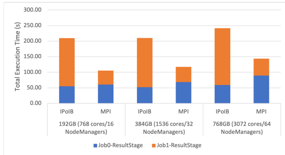
Fig. 9: GroupByTest weak-scaling performance numbers on Stampede2. The experiments were run on YARN cluster sizes of 16, 32, and 64 NodeManagers .
