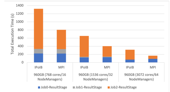
Fig. 12: SortByTest strong-scaling performance numbers on Stampede2. The experiments were run on YARN cluster sizes of 16, 32, and 64 NodeManagers .
