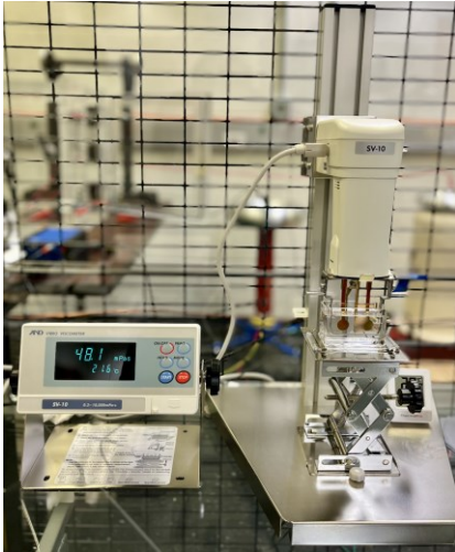
Fig. 1. Viscosity measurement of DBT at room temperature.
