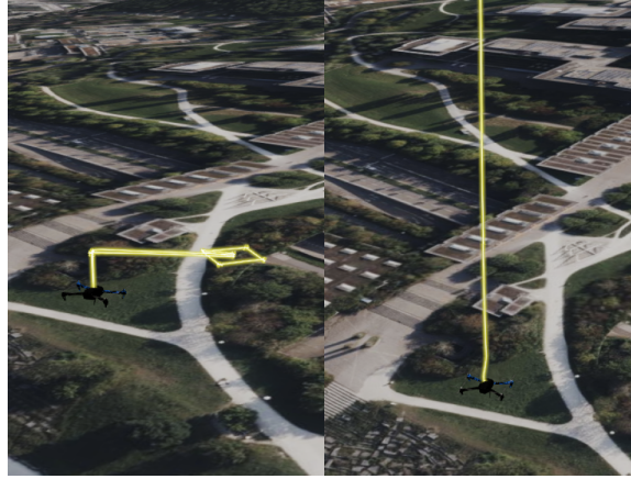
Fig. 7. Comparison of expected mission flight path (left) with rapidly ascending flight behavior (right) caused by pairwise misconfigurations.
