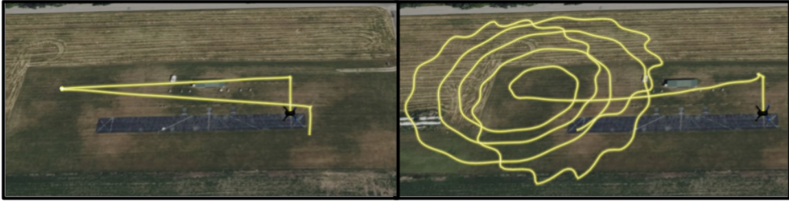
Fig. 8. Simulation results comparing the intended flight path for this mission with correct parameter tuning (left) versus the flight path observed in simulation without the benefit of adaptation when a faulty parameter value of MC\_ROLL\_P = 0.0 (right) was injected.
