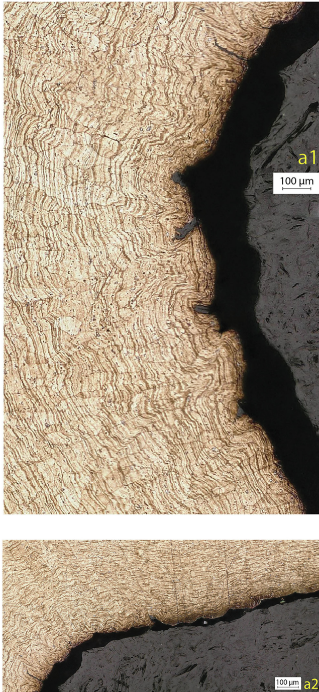
Fig. 9a. Expanded images of zones “a1” and “a2” from the overall image of tube from Exp. II in Fig. 4. Part of zone “a2” that is less bent shows surface wrinkles, whereas the more bent left side shows more pronounced wrinkles separated by creases. The higher curvature of zone “a1” has caused more significant protruding undulations and creasing.
