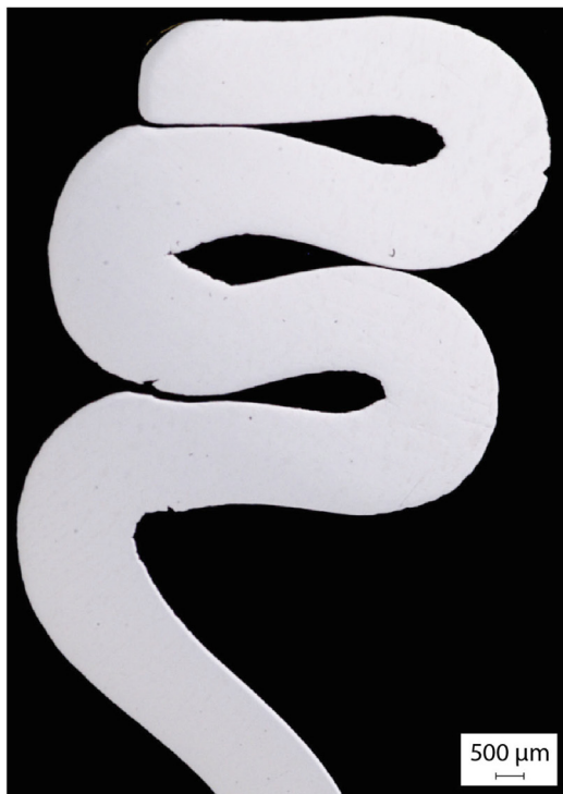
Fig. 1. (a) Crushed aluminum alloy tube exhibiting axisymmetric folding (Exp. II, D/t = 25.6 ). (b) Polished cross section of specimen in (a).
