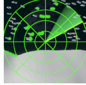
Fig. 4: The radar data are visualized through a minimap graphic in the bottom right of the screen. The green beam indicates the radar's current position, and the green dots are radar returns.
