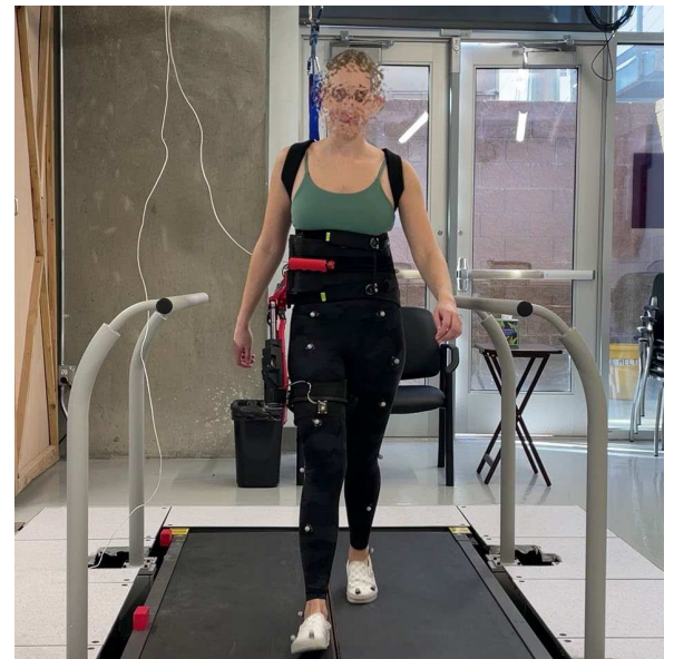
Fig. 3 Subject S1 walked on an instrumented treadmill with the powered exoskeleton in a unilateral configuration. Reflective marker trajectories were recorded with motion capture cameras. Ground reactions forces were recorded by the instrumented treadmill.
