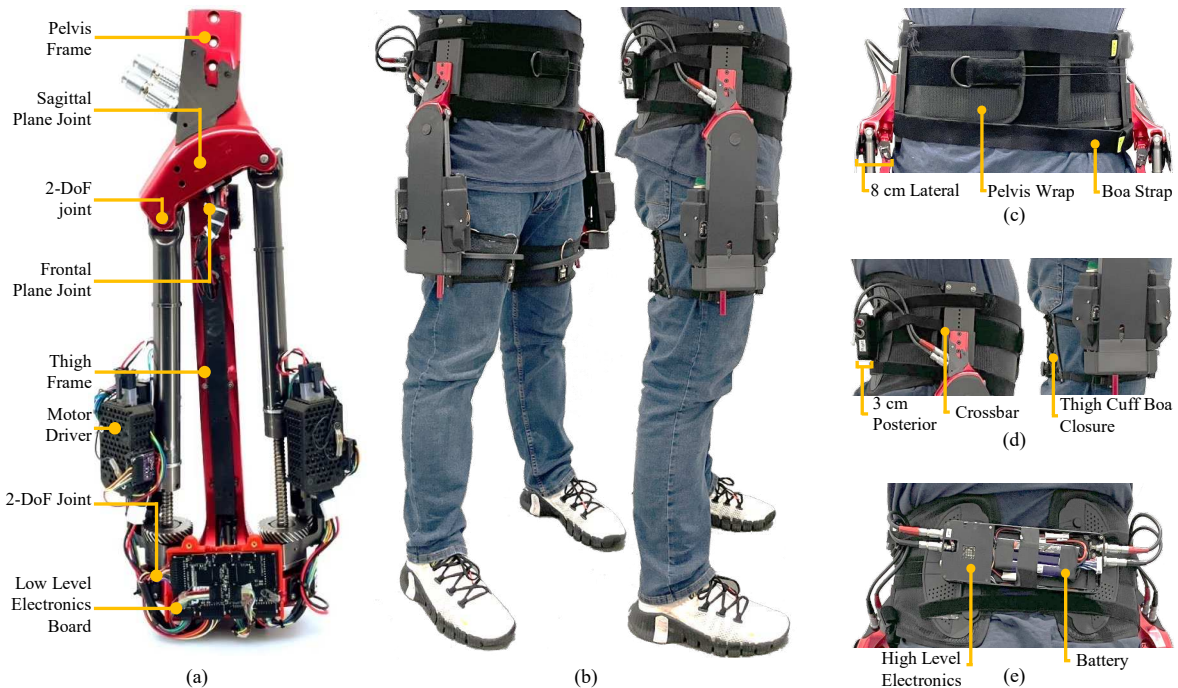
Fig. 1 (a) The hip actuator can generate flexion/extension and abduction/adduction torques. (b) The realized exoskeleton on a subject. (c-d) The hip actuator is connected to the subject's pelvis through a pelvis wrap with a rigid crossbar and to the subject's thigh through a rigid thigh brace with a flexible cuff. Both the pelvis wrap and thigh cuff can be tightened with a BOA closure system. (e) The high-level electronics and battery are placed posteriorly to the user. Per side, the hip actuator increases the user's lateral dimension by 8 cm. The high-level electronics and battery add 3 cm posteriorly to the user.
